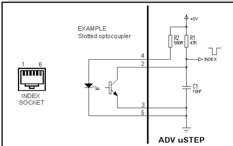
The circuit diagram shows how it is connected. AWR have a small circuit board with the correct connector and optocoupler on it using a standard RJ12 lead to connect to the INDEX connector.
