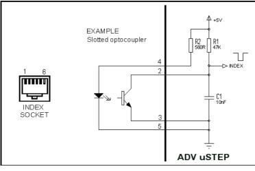
The circuit diagram shows how it is connected. AWR have a small circuit board with the correct connector and optocoupler on it using a standard RJ12 lead to connect to the INDEX connector.
