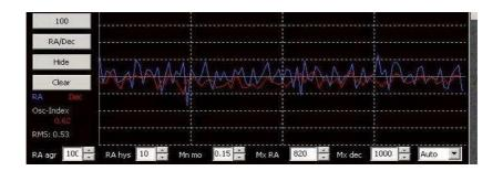
The graph – from PHD guiding, shows the RA and Dec traces after optimising with the PA2. NB. Lodestar has 8 micron pixels, astrograph is 1400mm fl, and the separation between dotted lines is one pixel.
